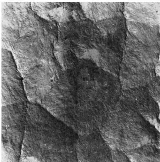
Fig. 13. Xylene-etched PEH. Ge-shadowed film, two-stage replica. ( \times 4000 )
