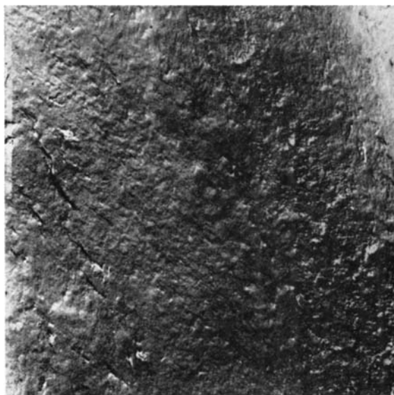
Fig. 14. Xylene-etched PEH-butadiene graft copolymer. Ge-shadowed film, two-stage replica. ( \times 4000 ).
